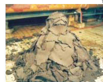
Sewage sludge from filter press and centrifuges
