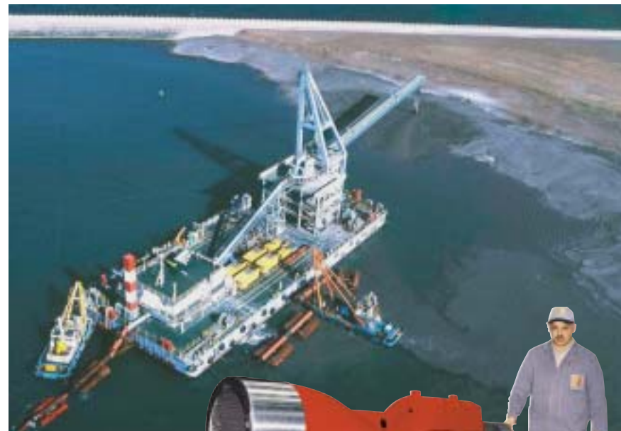
The largest S-pipe piston pump world-wide, manufactured by Putzmeister: KOS 25200 with a conveying performance of 550 m³/h. She is in operation claiming land just before Japan's coast
